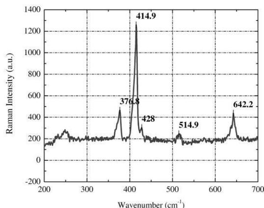
**Figure 1** Raman spectrum of the sapphire substrate.
