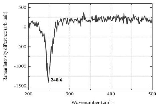
**Figure 4** Differential Raman spectrum of a-Se sample taken after 10 minutes illumination and 40 minutes relaxation respectively.
