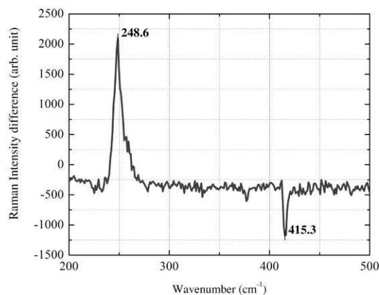
**Figure 3** Differential Raman spectrum of the non-illuminated and illuminated for 10 minutes a-Se samples.
