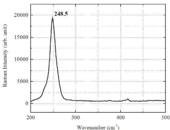
**Figure 2** Raman spectrum of non-illuminated a-Se sample.
