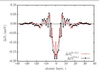
**Figure 5.** •: Calculated deviations in the layer-resolved MAE contributions,  $\Delta D_i^{(\mathrm{I_1I_1})}$ , of the composite stacking fault from the bulk Co MAE, see equation (6), and +: the corresponding average deviations,  $\Delta D_i^{(\mathrm{I_1+I_1})}$ , of two superposed  $\mathrm{I_1}$  type stacking faults centred on atomic layers  $i \pm 2$ , see equation (7). Solid lines serve as guides for the eyes.
