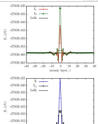
**Figure 1.** The layer-resolved contributions to the total energy in four hcp cobalt systems, each exhibiting one of the four different types of stacking fault. The label 0 refers to the plane of mirror symmetry. Solid lines serve as a guide for the eyes.
