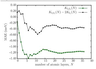
**Figure 6.** ★: Change in the MAE of hcp Co due the composite stacking fault,  $K_{I_1I_1}(N)$ , as defined in equation (8). •: Interaction term of the two stacking faults in the MAE,  $K_{I_1I_1}(N) - 2K_{I_1}(N)$ , see equations (4) and (8). Solid lines serve as guides for the eyes.
