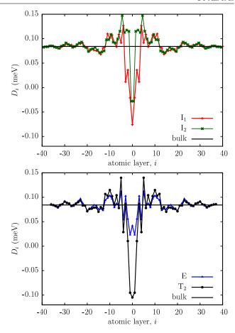
**Figure 3.** Calculated layer-resolved contributions to the MAE for stacking faults  $I_1$  and  $I_2$  (upper panel) and E and  $T_2$  (lower panel). The horizontal line refers to the bulk MAE, 84.4  $\mu eV/atom$ . Solid lines serve as guides for the eyes.
