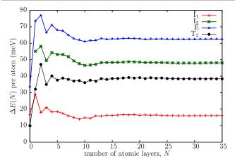
**Figure 2.** The cell-like part of the formation energy,  $\Delta E_X(N)$ , see equations (1) and (2), of stacking faults  $I_1$ ,  $I_2$ , E and  $T_2$  in hcp cobalt, displayed as a function of the number of layers, N, considered in the system on either side of the stacking fault. Solid lines serve as guides for the eyes.
