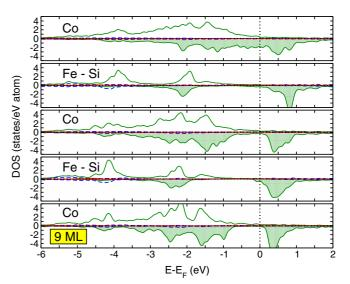
FIG. 20. (Color online) DOS of the Pt-Co<sub>2</sub>FeSi-Pt system with 9 monolayers of Heusler between the Pt leads.
