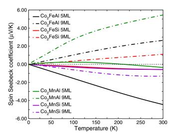
FIG. 16. (Color online) Comparison of the temperature dependence of the spin Seebeck coefficient of all systems under consideration.
