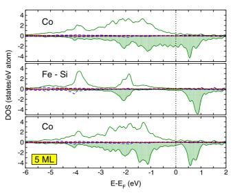
FIG. 19. (Color online) DOS of the Pt-Co<sub>2</sub>FeSi-Pt system with 5 monolayers of Heusler between the Pt leads.
