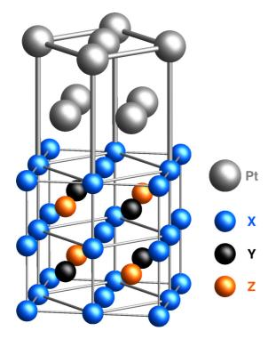
FIG. 1. (Color online) Schematic view of the interface between Pt leads and Heusler layers. The Pt lattice is rotated with respect to the Heusler lattice because the length of the diagonal of the Pt lattice is comparable to the lattice constants of the Heusler alloys. This ensures that the lattice mismatch between both metals is between 0.06 and 0.11 Å.
