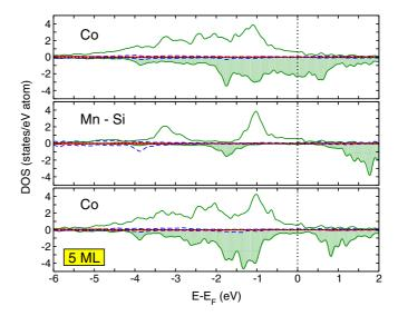
FIG. 23. (Color online) DOS of the Pt-Co<sub>2</sub>MnSi-Pt system with 5 monolayers of Heusler between the Pt leads.
