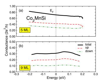
FIG. 15. (Color online) Energy dependence of the conductance of the Pt-Co<sub>2</sub>MnSi-Pt system with 5 and 9 monolayers of Heusler around the Fermi energy.
