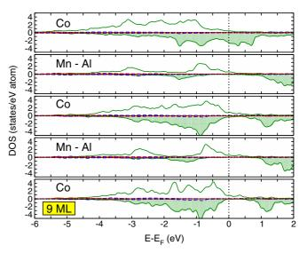
FIG. 22. (Color online) DOS of the Pt-Co<sub>2</sub>MnAl-Pt system with 9 monolayers of Heusler between the Pt leads.
