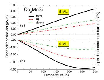
FIG. 14. (Color online) Temperature dependence of the Seebeck coefficient of the Pt-Co<sub>2</sub>MnSi-Pt system with 5 and 9 monolayers.
