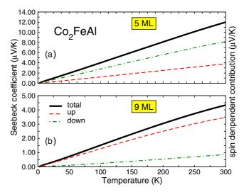
FIG. 8. (Color online) Temperature dependence of the Seebeck coefficient of the Pt-Co<sub>2</sub>FeAl-Pt system with 5 and 9 monolayers. The black line denotes the total Seebeck coefficient and the green and red lines denote the contributions from the two spin channels according to the color coding used for the energy dependence of the conductance.
