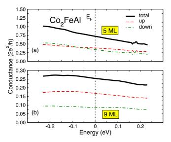
FIG. 9. (Color online) Energy dependence near the Fermi energy of the conductance of the  $Pt-Co_2FeAl-Pt$  system with 5 and 9 monolayers. The black line denotes the total conductance, whereas the green and red lines denote the contributions from the two spin channels.
