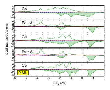
FIG. 18. (Color online) DOS of the Pt-Co<sub>2</sub>FeAl-Pt system with 9 monolayers of Heusler between the Pt leads.
