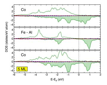
FIG. 17. (Color online) DOS of the Pt-Co<sub>2</sub>FeAl-Pt system with 5 monolayers of Heusler between the Pt leads. Here and in the following 7 figures, green lines and shaded areas show layer-resolved projections on the 3d orbitals of the denoted layer, while red solid and blue dashed lines depict summed-up projections on the valence s and p orbitals, respectively.
