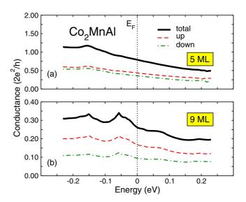
FIG. 13. (Color online) Energy dependence of the conductance of the  $Pt-Co_2MnAl-Pt$  system with 5 and 9 monolayers of Heusler around the Fermi energy.
