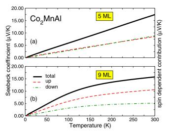
FIG. 12. (Color online) Temperature dependence of the Seebeck coefficient of the Pt-Co<sub>2</sub>MnAl-Pt system with 5 and 9 monolayers of Heusler.
