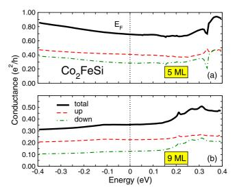
FIG. 11. (Color online) Energy dependence of the conductance of the  $Pt-Co_2FeSi-Pt$  system with 5 and 9 monolayers of Heusler around the Fermi energy.
